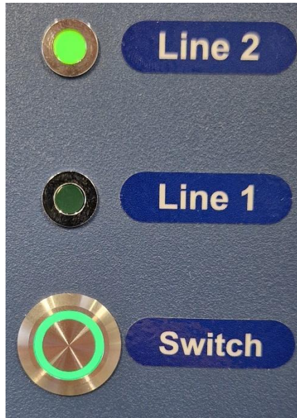
Figure 20.4 The MIRI® TL12 multiroom IVF incubator's line altering switch and an active Line 2
