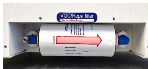
Figure 12.3 Correctly installed VOC/HEPA filter
