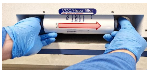
Figure 12.2 VOC/HEPA filter insertion and removal procedure
